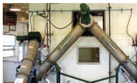
Two auger conveyors converge
